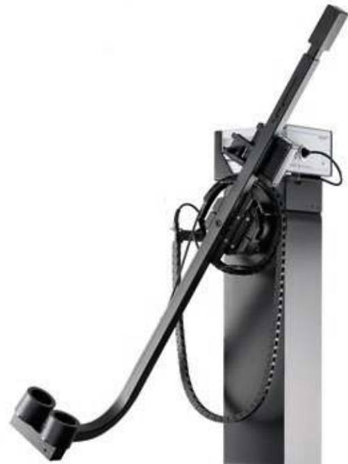
Luminous flux integrator with photometer and spectroradiometer
