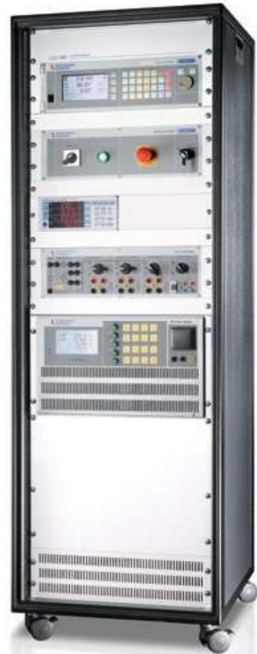
Rack with control unit, power supply for the test specimen and power meter
