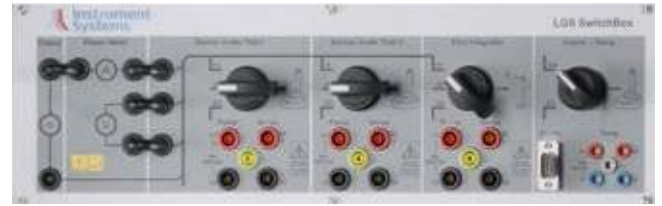
LGS SwitchBox for connecting to the sample supply terminal
