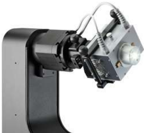
Sample holder with LED-850 test adapter for single LEDs
